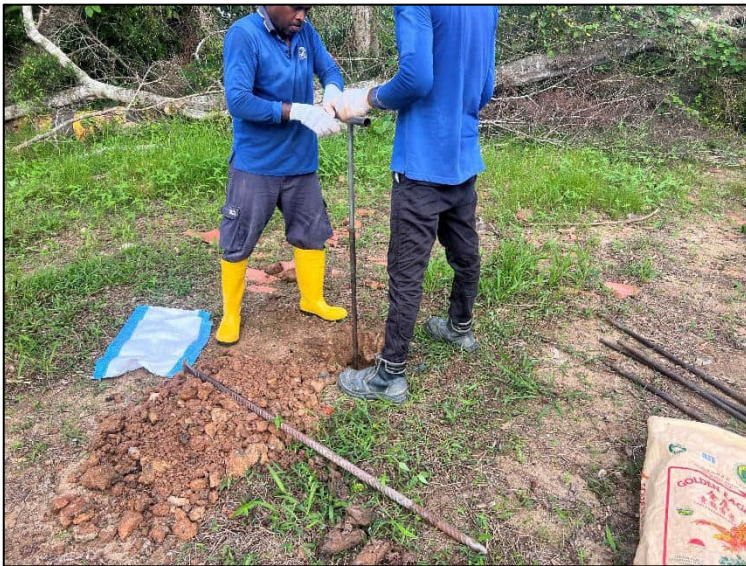
Figure 9-1 Soil boring (TC-BH02)
